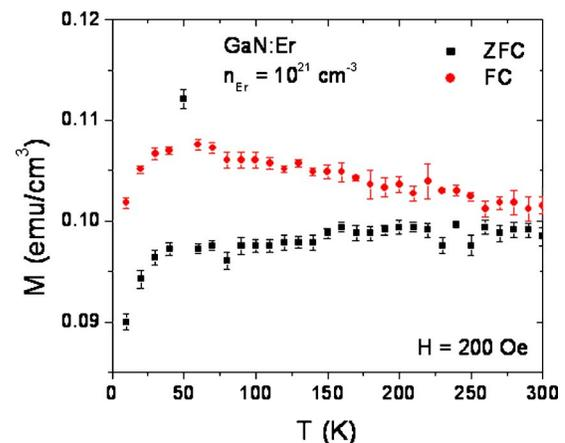
FIG. 3. SQUID measurements as a function of temperature from GaN epilayer with an Er concentration of  $\sim 10^{21}\text{ cm}^{-3}$ , in an applied field of 200 Oe. Field-cooled and zero-field-cooled magnetization data points are shown.
