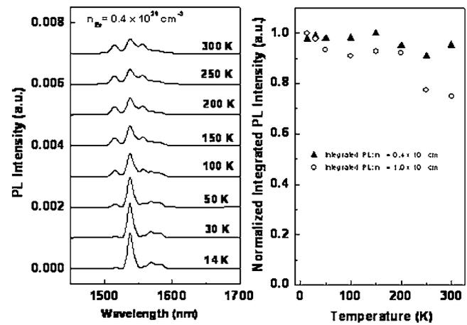
FIG. 2. (a) PL spectra at indicated temperatures taken from the epilayer having an Er concentration of  $\sim 4 \times 10^{20}\text{ cm}^{-3}$ ; (b) Thermal quenching of the integrated PL intensity for samples with  $n_{\text{Er}}$  of  $0.4 \times 10^{21}\text{ cm}^{-3}$  and  $1.0 \times 10^{21}\text{ cm}^{-3}$ .
