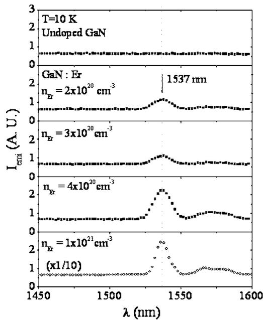
FIG. 1. Infrared PL spectra taken at 10 K from GaN epilayers having Er concentrations in the range of  $(2\text{--}10)\times 10^{20}\text{ cm}^{-3}$ . PL from an undoped control sample is also shown.
